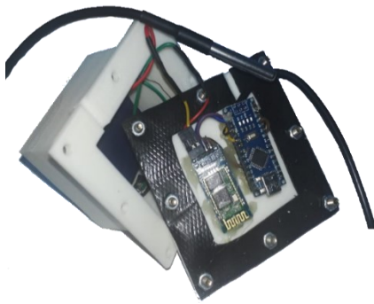
Figure 12 Prototype of embedded wireless maturity sensor and its features
